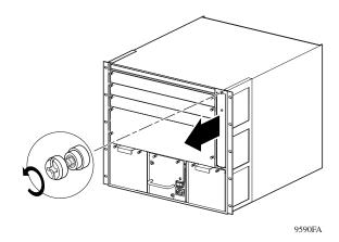
1. Loosen the retaining screws and pull the fan tray out of the chassis until the power connector disconnects from the backplane.
